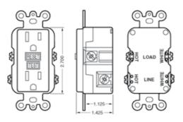
Figure 1: GFCI Layout
